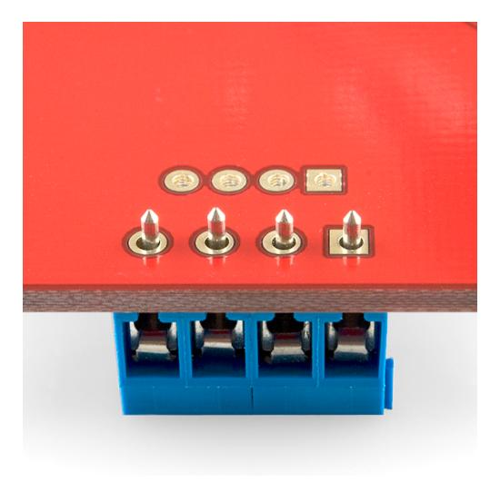
Now, while holding the screw terminals with your thumb, turn the board over and place it on the table so that the screw terminal pins are sticking out the other side of the board. Don't worry about crooked pins at this point, we'll take care of that.
