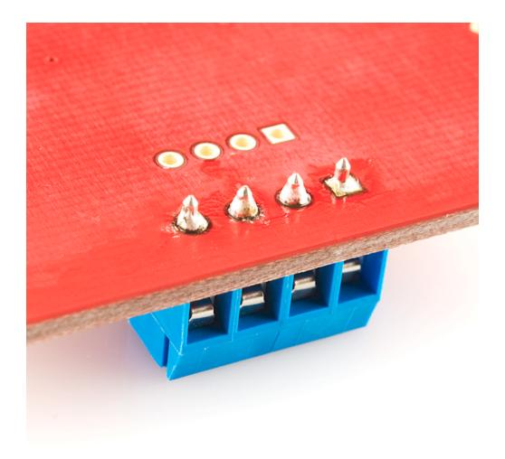
Now onto the headers. The kit comes with stackable headers, but you may alternately want to install regular male headers if you're not going to be stacking anything on top of the Ardumoto and save the stackables for another project. For the purpose of this tutorial, we'll go with the stackables since they're more difficult to install.
